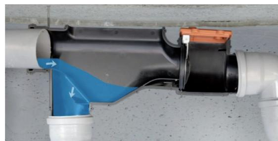
High rainfall events, that occur approx. 4 to 10 times in a year, contribute only about 3% to total water yield and are used by the PURAIN Rainwater filter for self-cleaning. These high rainfalls lead to the formation of an eddy in the PURAIN rainwater filter, the so called hydraulic jump, which spins with such great force that even dirt accumulated in the tray is flushed and discharged with the overflow.
